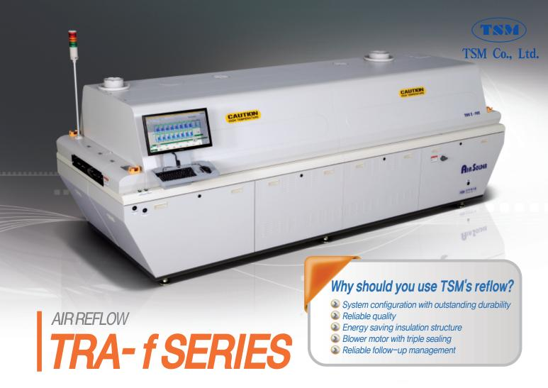
The TRA series reflows are an innovative design that ensures efficient flux discharge as well as highly efficient thermal management
